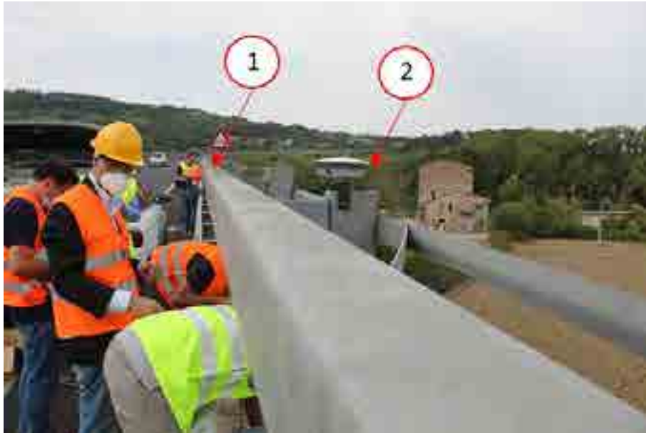
Figure 83. View of the antennas installed in the first (in background) and the second monitored point (in foreground).
