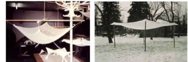
(a) Hanging cloth model (b) Hanging cloth model left to freeze
