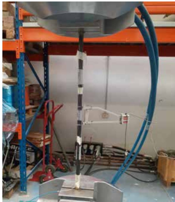
Figure 22. Extensometer positioning for direct strain measurement
