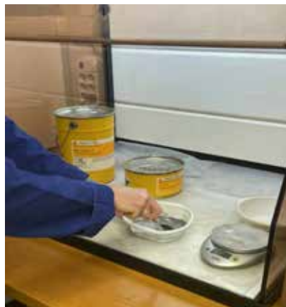
Figure 12. Production of the SIKADUR 330 epoxy resin.
