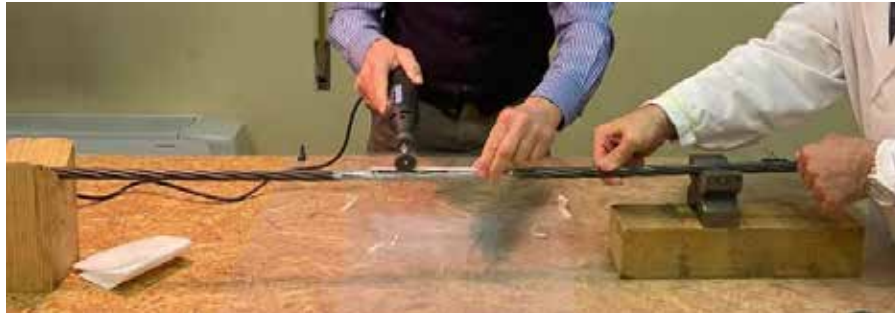
Figure 18. Cutting a small part of smart saddle after curing.
