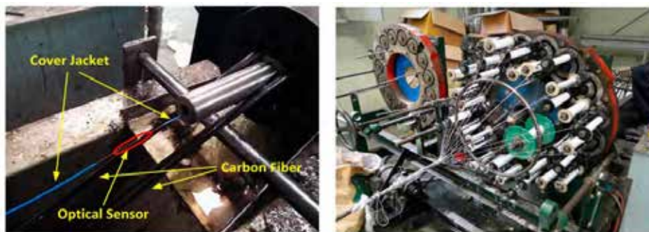
c) Replacing inner steel wire with carbon fiber with embedded FBG (S. T. Kim et al., 2015)
