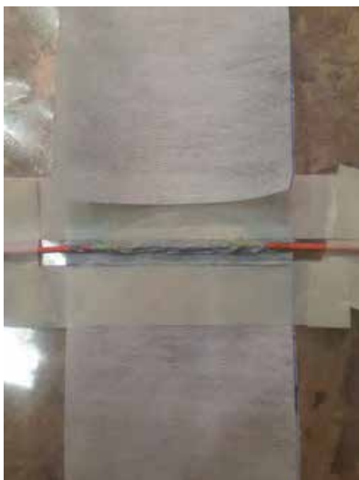
a) FBG + coating gluing to polyester paper
