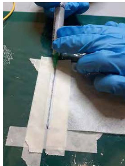
b) Add two extra scotch tapes and epoxy resin
