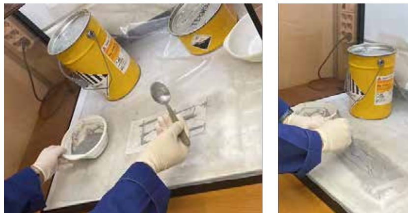
Figure 13. Putting the mixed epoxy resin on the both side of Polyester.
