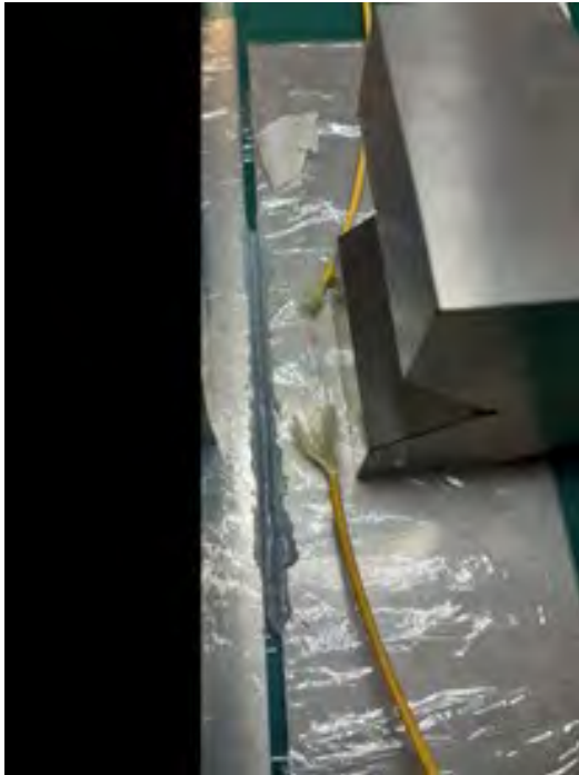
d) Apply a thin line of epoxy and positioning fiber on the groove
