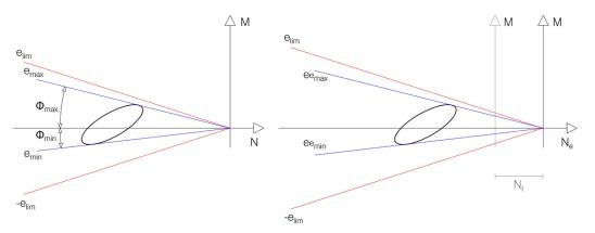
Left: Ellipse of eccentricity or RF ellipse. The generalized eccentricity extrema ( $e_{\max}$ ,  $e_{\min}$ ) are equal to the slopes of the blue lines. The admissibility domain ranges between  $e_{\lim}$  and  $e_{\lim}$ , which are the slopes of the red lines.  $\Phi_{\max} = \arctan(e_{\max})$  and  $\Phi_{\min} = \arctan(e_{\min})$  are the eccentricity angles.
