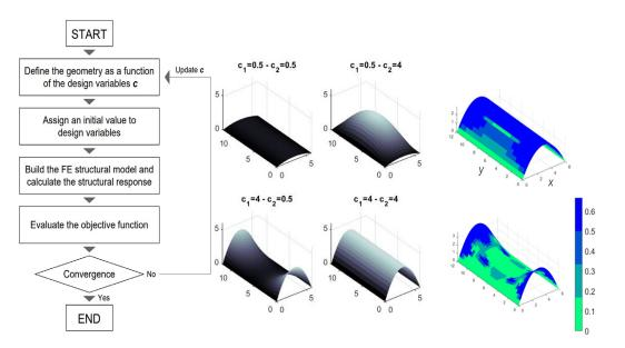
Left: Main steps of the R-Funicularity based shape optimization process
