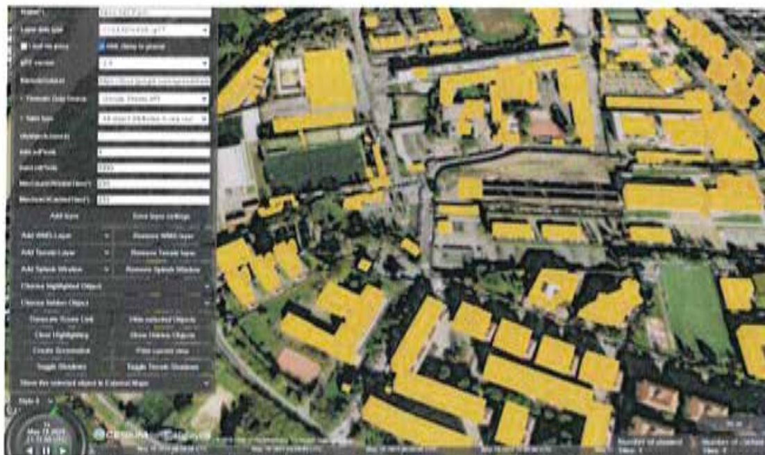
Fig. 3. 3D visualization in Web Map Client (interface for 3DCityDB based on Cesium JS) of an initial set of buildings in the Valco San Paolo area, obtained from the CityGML database through an export in the specified format.
