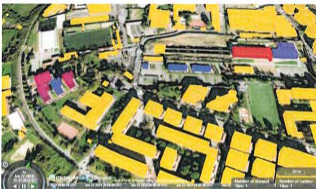
Fig. 8. Execution in 3D Web Map Client of a script for conditional coloring of buildings. A graphical representation of the cooling power demand for summer air conditioning is shown for a selection of buildings at Roma Tre University (colors range from blue to red).
