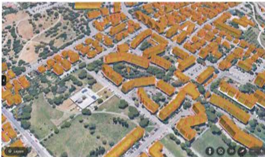
Fig. 1. Results of importing a dataset on Cesena into CityGML, extracted from the Regional Topographic Database of Emilia-Romagna. The images show the 3D component visualized in Google Earth through KML format export.
