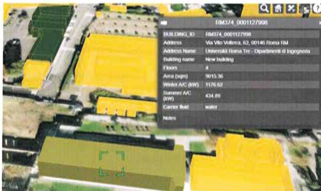
Fig. 7. 3D visualization in Web Map Client of metadata read in real-time from a linked document (in this case, a Google Sheets document).
